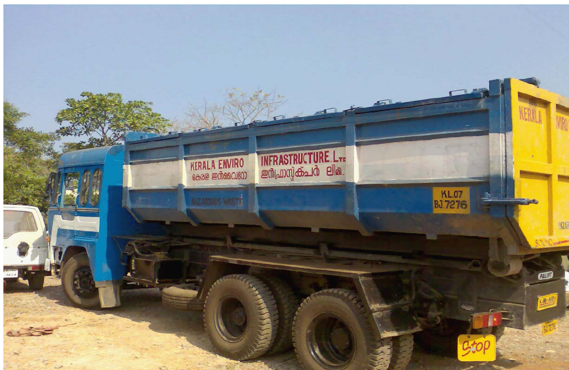
Figure 5.1. special purpose vehicle for transportation of hazardous waste
